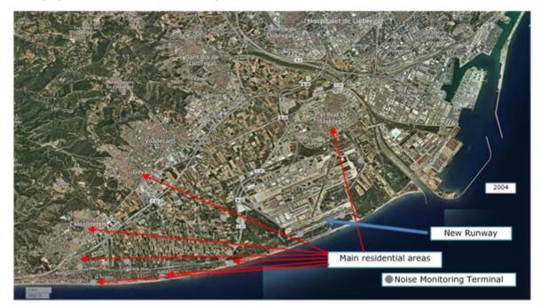
The new infrastructure is equipped with the maximum category runway lighting facilities (ILS Category II/III systems in each departure point). This enables its use in both directions and in foggy conditions. Runway 07L-25R has also been lengthened to 3,743 m and widened to 60 m.
