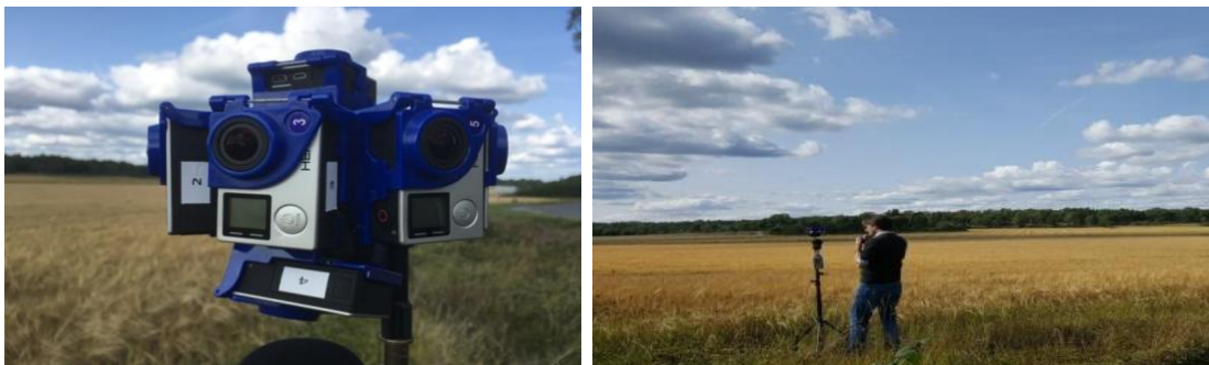
Figure 5: Setup for 360-degree video recordings of the environment and the aircraft movements
